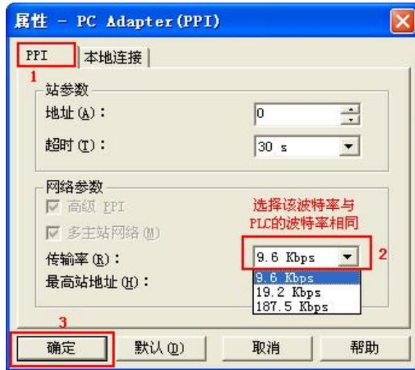
4. Online test: After USB Adapter CN connects RS485 interface of S7-200CPU and USB port of PC, click the “communicate” button in the lower left corner of main interface to enter searching PLC interface, double-click “Double-click Refresh” icon, then you can search out the PLC which is connected with USB Adapter CN, Select the PLC and then click “OK” to return the main interface. Now you can go on the work such as program download and upload, monitoring etc.
