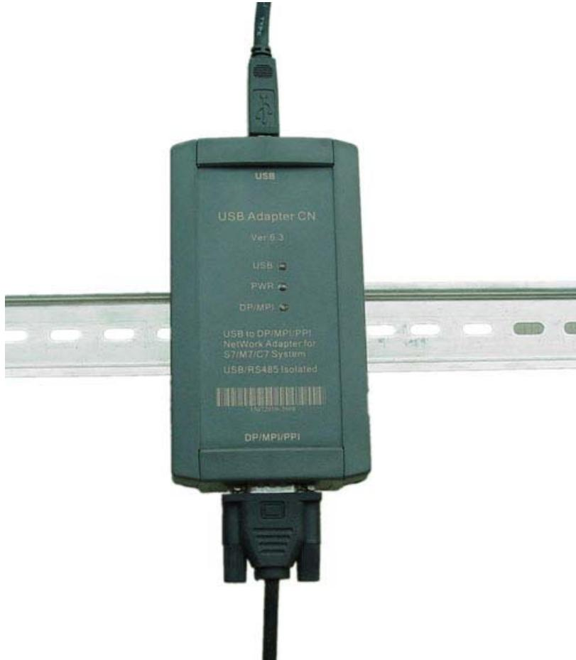
USB Adapter CN has been installed on the standard rail
