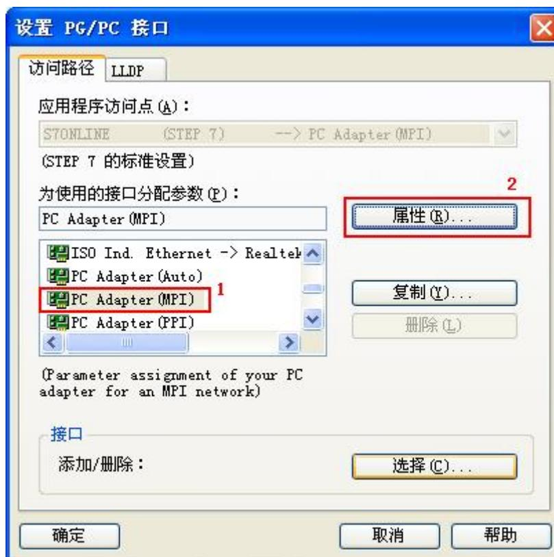
2.Click the top “MPI” option,set the adapter MPI interface parameter,choose the baud rate 187.5Kbps or 19.2Kbps or 1.5Mbps,this baud rate must be the same as the PLC MPI interface baud rate.If you don’t know the PLC MPI interface baud rate,you could choose “PC Adapter (Auto) ” to check.Other parameters are default,click “OK” button to return the previous menu,click”OK” to return the main interface.
