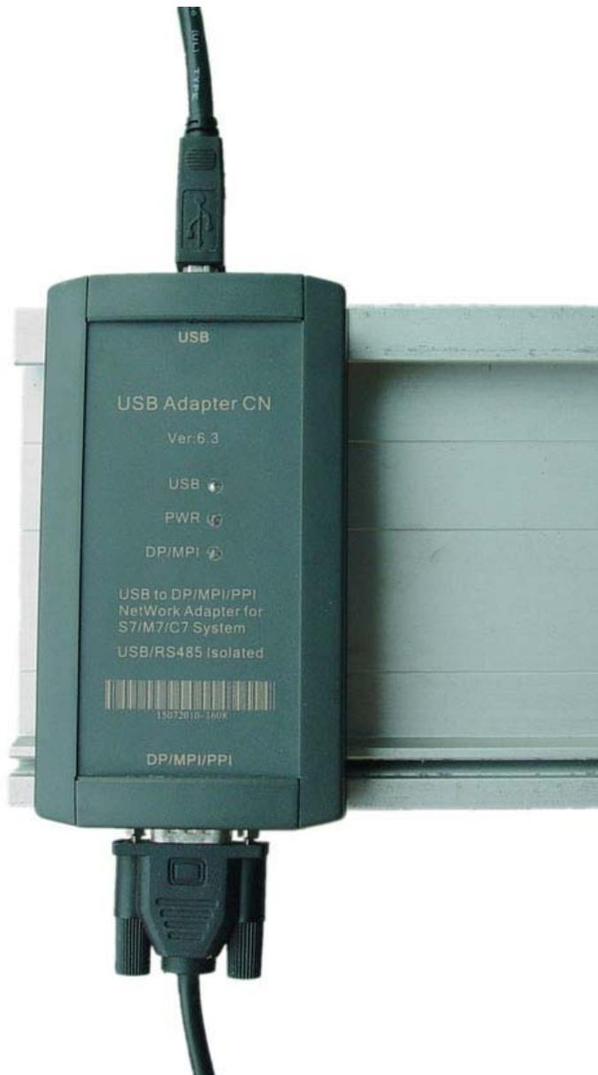
USB Adapter CN has been installed on the S7-300PLC rail
