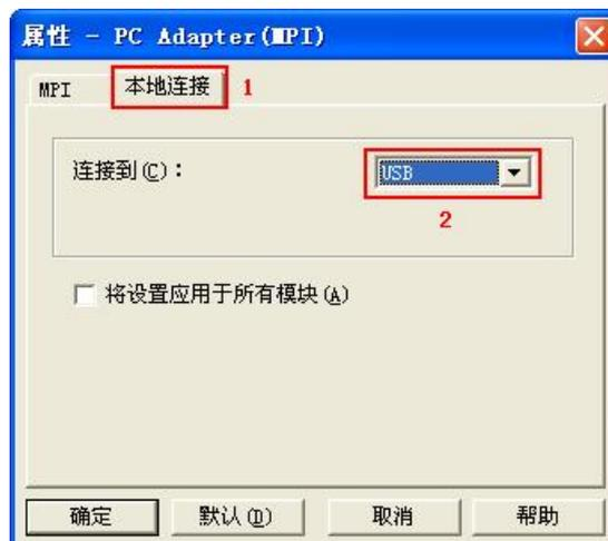
In the next the connection between USB Adapter CN and DP/MPI/PPI interface of PLC is OK,and you could do the downloading,uploading and monitoring operation.
