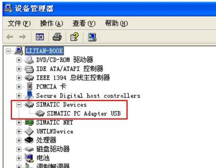
It will appear the “USB” option in the “local connection” of “set PG/PC interface” in the Step7 software after you finish installing the driver, and then choose this USB option.
